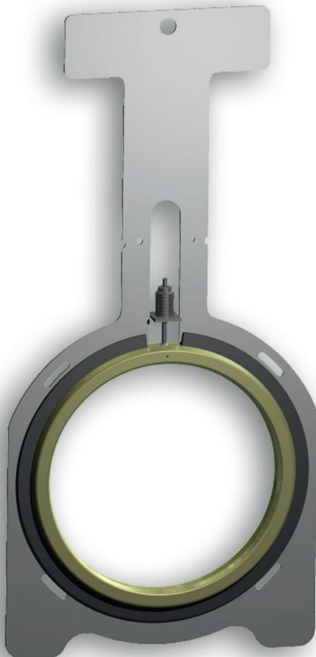
The KGIT decreases the risk of injury to divers' hands and fingers as the engineered profile is designed to locate accurately within the lower bolts of the flange, ensuring the gasket sits correctly in the groove. With well positioned holes designed to accommodate standard subsea tooling, the KGIT aids transportation and fitting. Flange alignment tools can be left in the flange as the gasket is fitted minimising movement of the flanges ensuring there is no 'bruising' or 'pinching' to the gasket.
