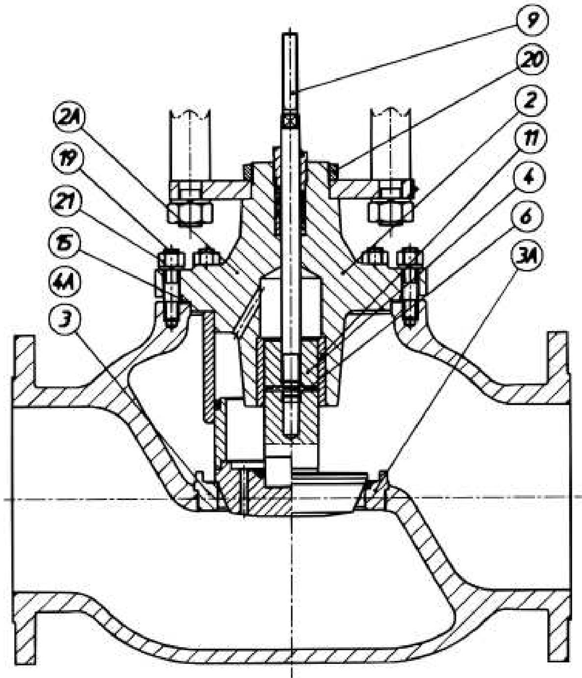
Figure 3 – Regulator valves DN 150... 250 with valve block Kvs = 63... 630
