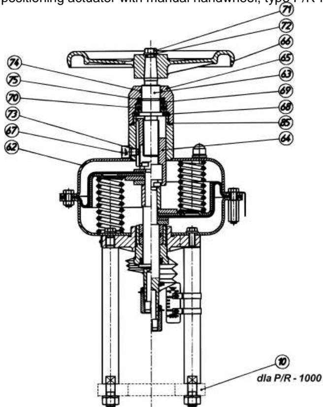
Figure 5: Manual actuator, type NN
