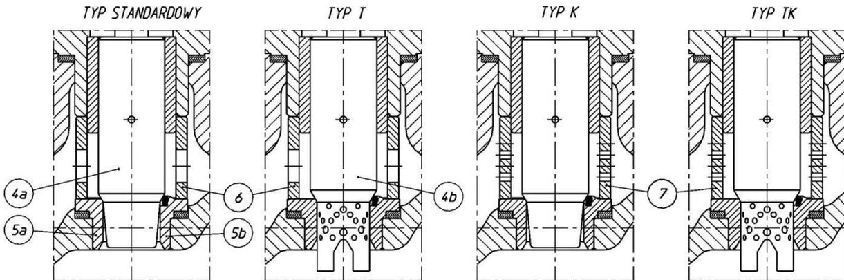
Figure 3: Different models of control valve type BR12a
