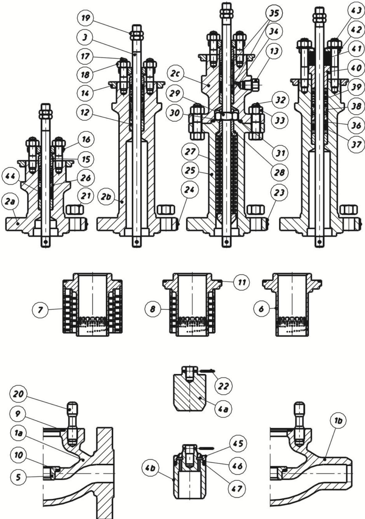
Figure 3: Pneumatic positioning actuator with manual handwheel, type P/R-N
