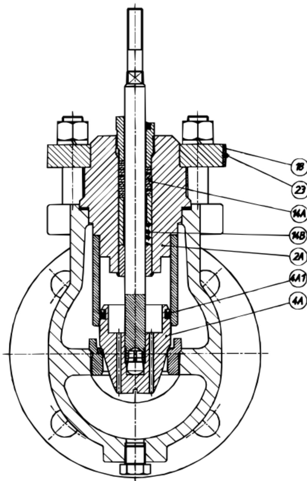
Figure 2 – Regulator valve DN 40... 100 with pressure-balanced block
