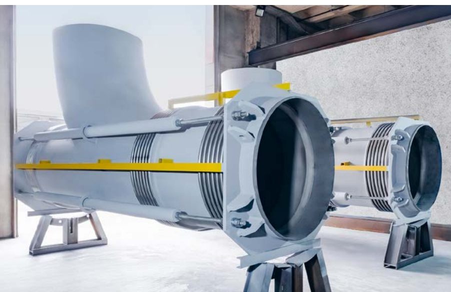
Custom expansion joints being prepared for Dradenau.
