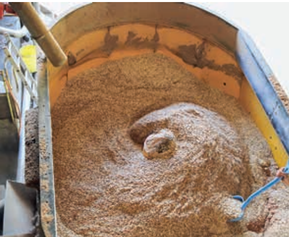
Up to four tons of mushroom cultivation substrate made mainly of beech sawdust is mixed and heated in the agitator.
