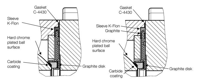
For abrasive media and media containing solids, as well as for media that are heavily contaminated and granular or have a tendency to crystallize.
