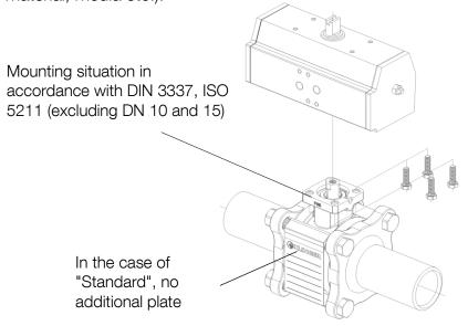
Direct mounting of an actuator (as illustrated in the image above) is only recommended for operation temperatures under 80 °C.
