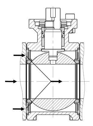
This principle is used in combination with ball valves of smaller nominal sizes. As the nominal sizes increase, so do the forces which have to be absorbed by the sealing rings. In order to achieve a long service life and to keep the torques for the pivoting of the ball as low as possible, this three-component design is not suitable for all nominal sizes.
