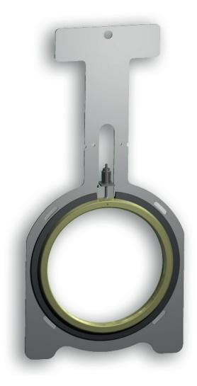
The KGIT decreases the risk of injury to divers' hands and fingers as the engineered profile is designed to locate accurately within the lower bolts of the flange, ensuring the gasket sits correctly in the groove. With well positioned holes designed to accommodate standard subsea tooling, the KGIT aids transportation and fitting. Flange alignment tools can be left in the flange as the gasket is fitted minimising movement of the flanges ensuring there is no 'bruising' or 'pinching' to the gasket.
