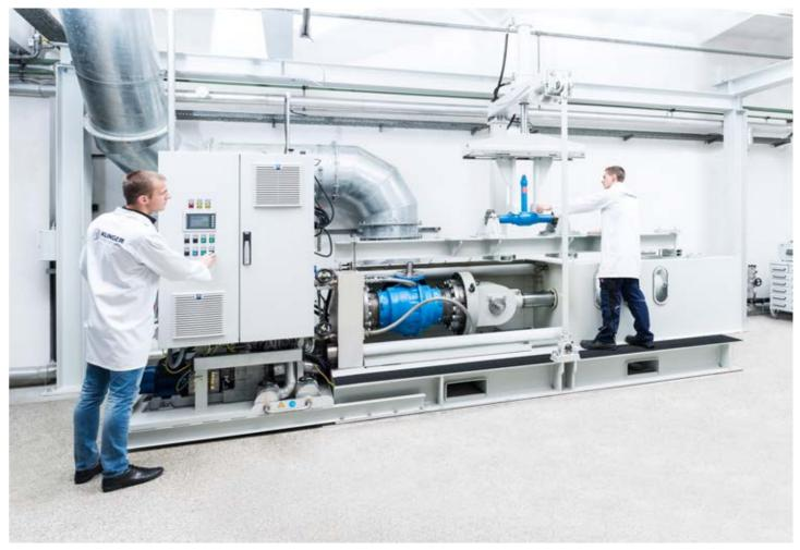
EN 488 defines the technical requirements as well as the testing procedure for underground shut-off valves integrated directly into the district heating network.
