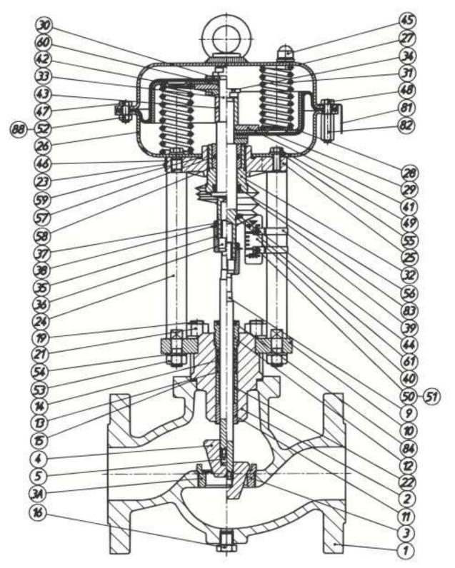
Figure 1 – Regulator valve DN 15... 100 with valve plates Kvs = 25... 160, with pneumatic positioning drive
