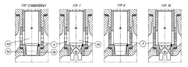
Figure 2: Different types of valve plug and pressing cages
