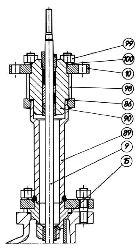
Figure 6 – Model with extended cover
