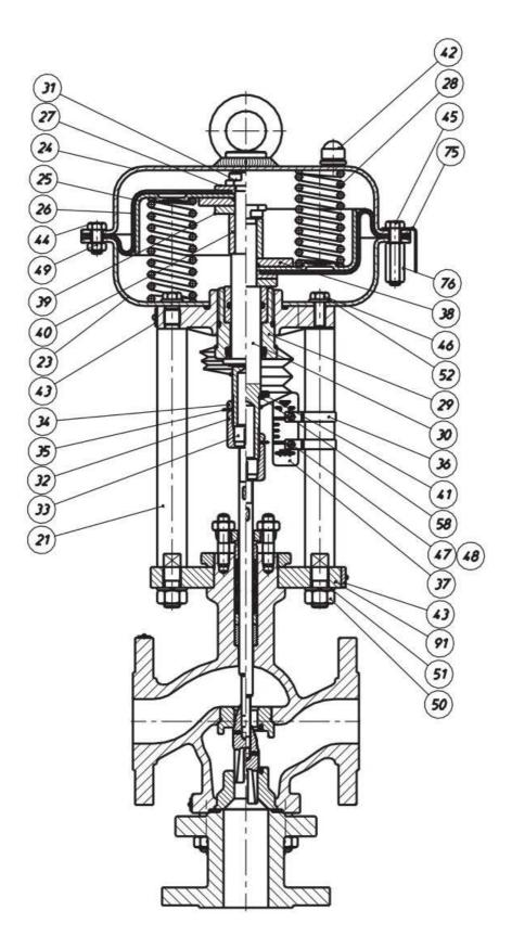
Figure 2a Valve BR13 with pneumatic drive P/R
