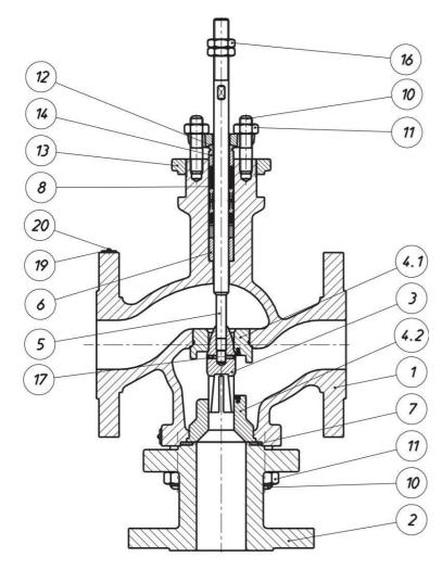
Figure 1a valve BR13 with standard stuffing box
