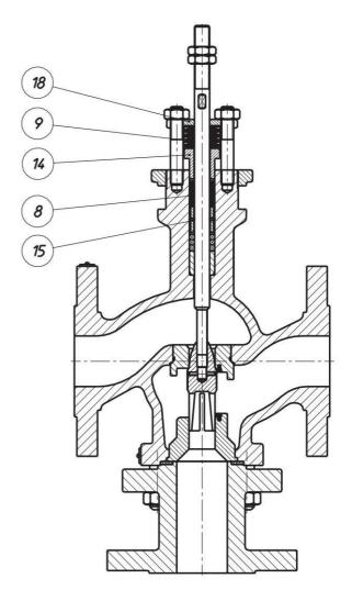
Figure 1b Valve BR13 with TA-Luft stuffing box
