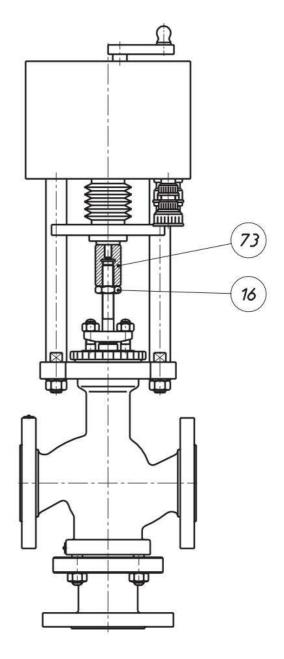
Figure 3b Valve BR13 with electric drive
