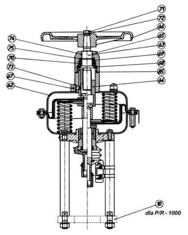
Figure 8 - Pneumatic positioning drive with manual drive type P/R-N
