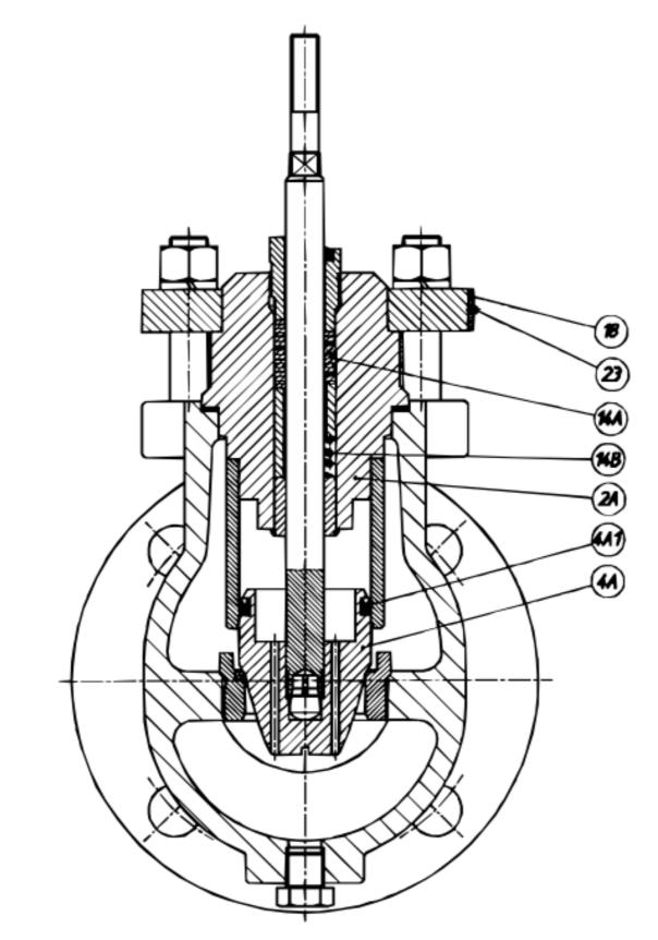
Figure 2 – Regulator valve DN 40... 100 with pressure-balanced block
