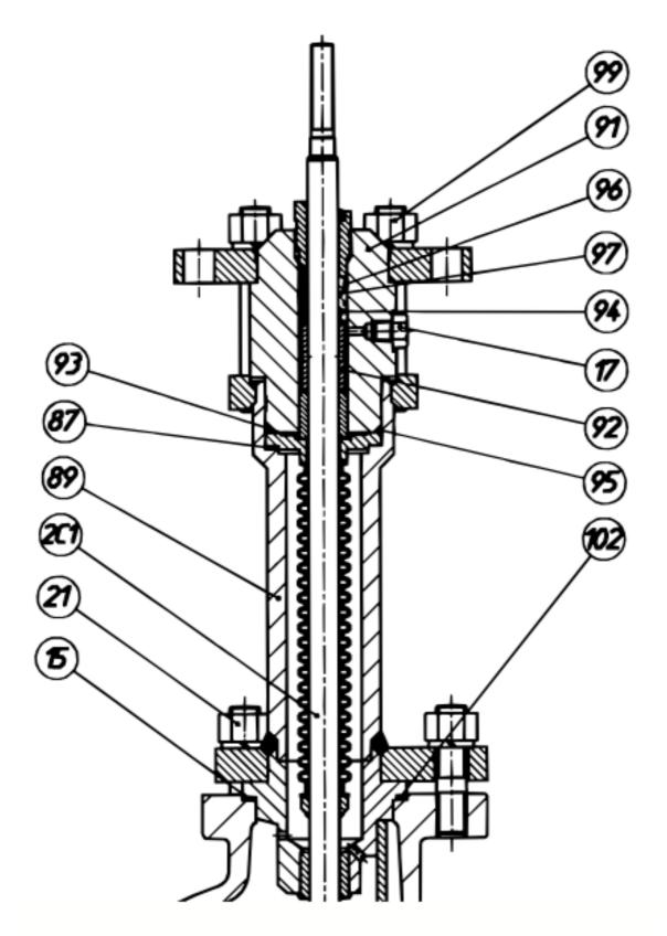
Figure 7 – Model with bellows - 2C
